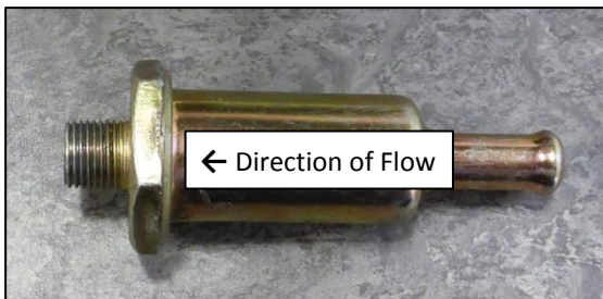
Photo No. 6: Fuel filter as removed
