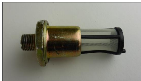
Photo No. 7: Fuel filter exposed and found to be free from debris
