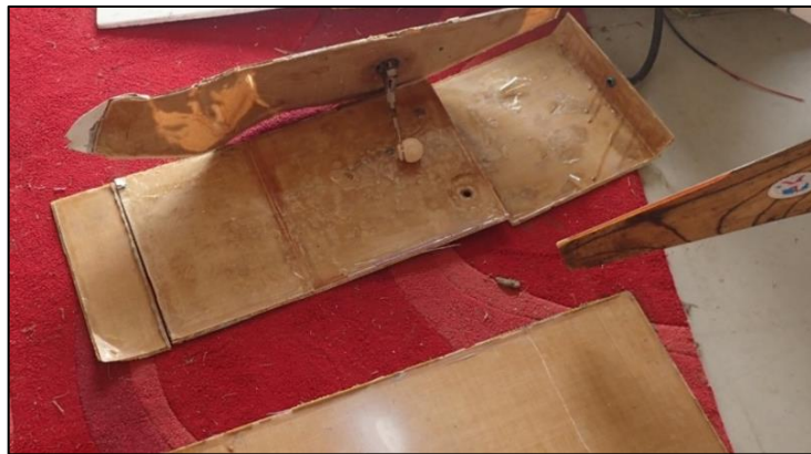
Photo No. 2: Slipper tank separated into its constituent flat panels
